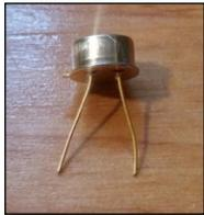
**Figure 1.** Photo of a Nanolog Device in a TO can format. Cans numbered 1-25 are N1 devices, while 26-50 are N2, corresponding to the IV curves in figure 2 below.
